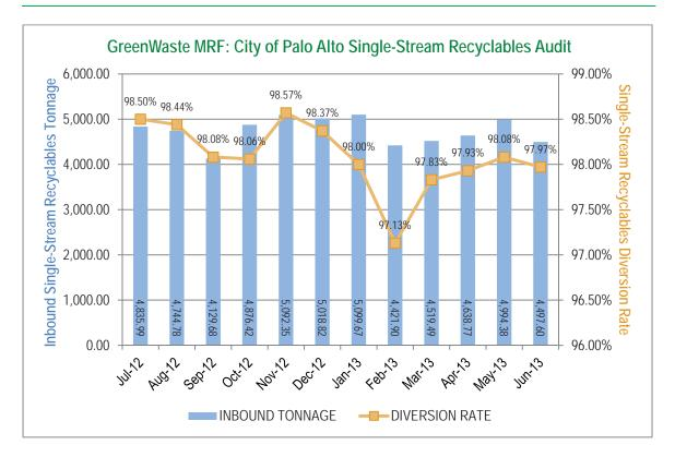
The GreenWaste MRF exemplifies innovative recovery facility processing operations. Since the upgrade to the facility in 2008, GreenWaste has performed numerous audits which consistently result in diversion rates of over 97%. GreenWaste commits to a diversion rate of at least 95% for the single-stream Recyclable Materials collected and processed for the Participating Agencies.
